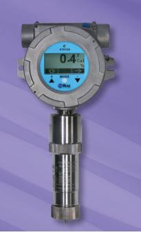
The RAEGuard 2 PID is a fixed photoionization detector (PID) that measures a broad range of volatile organic compounds (VOCs). The RAEGuard 2 PID operates on 10 to 28 VDC and provides an analog (4-20mA) three-wire signal output, and RS-485 Modbus digital signal output. Calibration and maintenance have been greatly simplified as the digital PID module can be easily removed in hazardous locations for calibration or maintenance.
